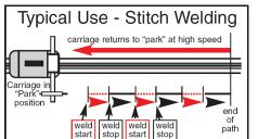
accessories (sold separately). It is ideal for stitch welding and seam welding applications where repeatability is desired. The reliability and precision of this automated welding and cutting system reduces cost, adds efficiency and improves
